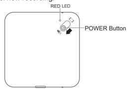
**POWER Button** (2) Switch the "RECORD" back to the middle position to stop recording and power off LED light will turn off.
